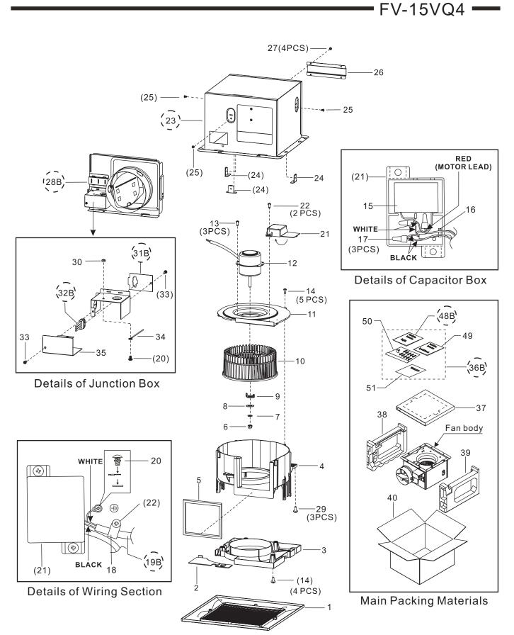
Remark: Because of different structure, we divide this model into Version A & Version B. In Version A, we also divide into Style A & Style B. The change points are mainly refer to the installation method and the cord section, please pay attention to the parts which circled with broken line, you can refer to the following 3 pages for details.
